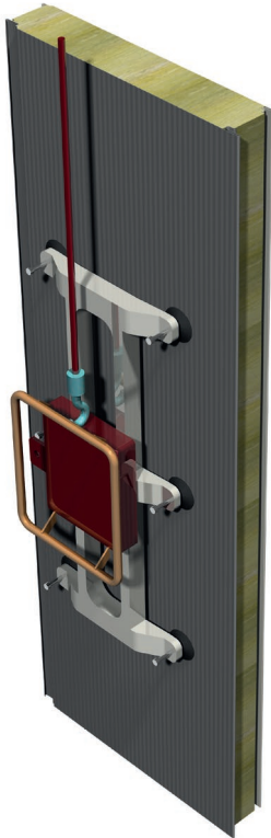
Fig. 49: Vertical lifting with mechanical gripper; Vertical lifting with vacuum gripper.
