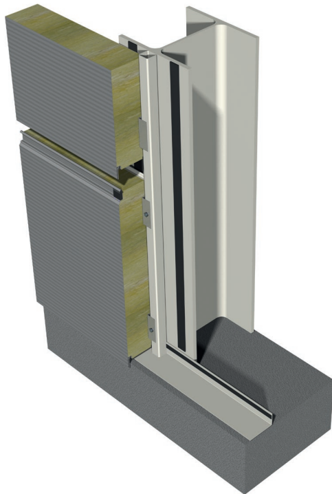
Fig. 34: Indirectly fixing back steel sheet into spacer
