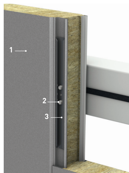
Fig. 4: Fixing in the light steel structure.
